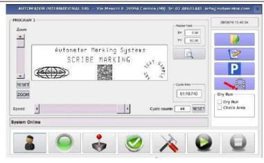
provides for the creation of messages with the date in various formats, fix or variable texts, codes, serial numbers, Datamatrix and logos. Possible the creation of the programs on the PC (running Windows operating systems), which can be easily transferred to the AC500 controller with USB stick or USB connection.
