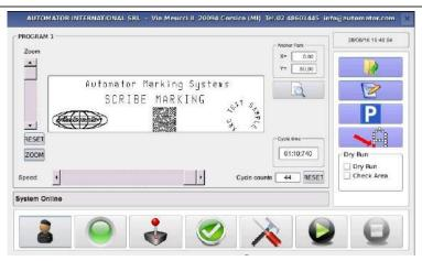
displayed instantly. The software provides for the creation of messages with the date in various formats, fix or variable texts, codes, serial numbers, Datamatrix and logos. Possible the creation of the programs on the PC (running Windows operating systems), which can be easily transferred to the AC500 controller with USB stick or USB connection.
